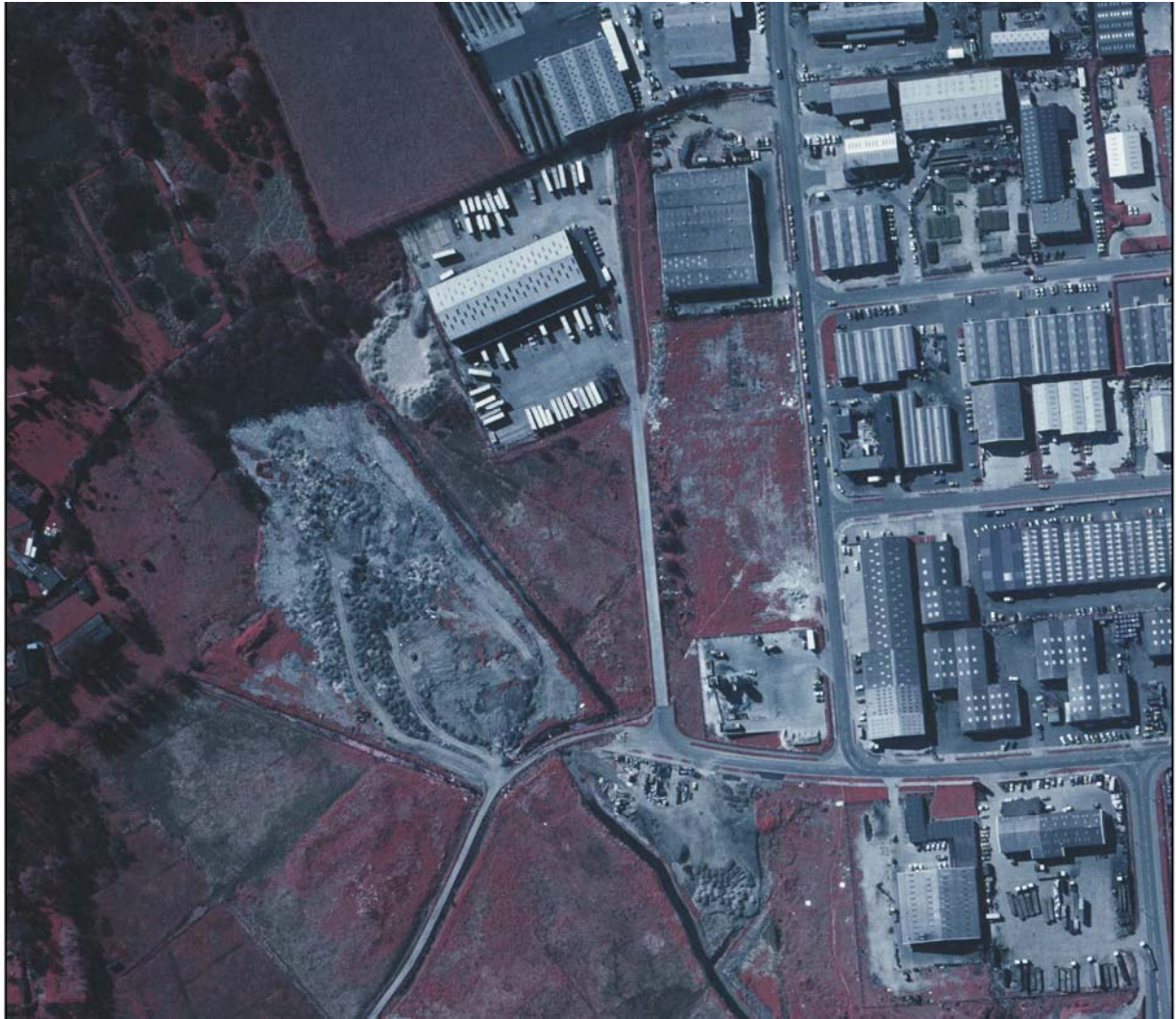
Figure 4. Example of colour infrared photography in an urban area. Nutrient rich grassland has most reflectance, and therefore has most colour. Nutrient stressed vegetation will be duller and more patchy at certain times of the year.
